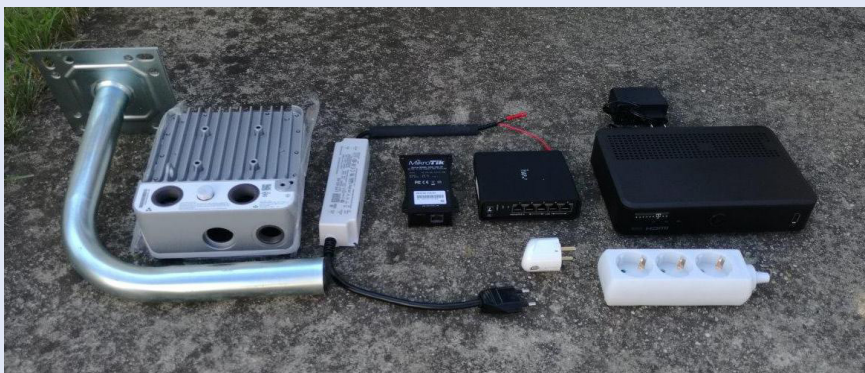
Figure 05 | All parts required for one installation: antenna mount, virtual fiber radio link, router, converter, power supply, IPTV STB for some customers, cable ducts and Ethernet cable, etc.
