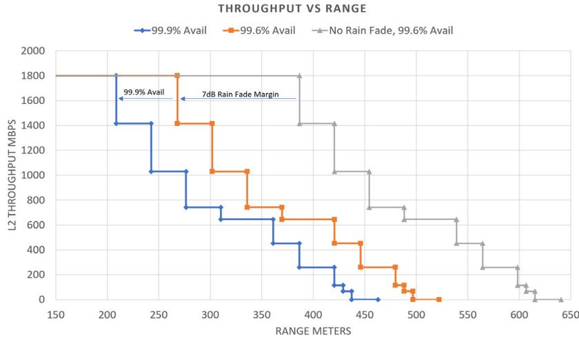
In field deployment link level availability varies on the above parameters and is measured by monitoring MTTF and MTTR.
