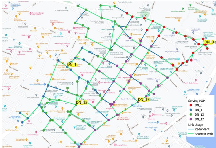
The plot above shows DN's with four different colors based on the serving POP. Each of the clusters operate independently while all the shortest path links are available. The moment a Shortest Path link fails, The network will start routing traffic to the nearest POP using the Redundant links. In case of a failure of a POP, the traffic in a cluster will get routed to other available POP's.
