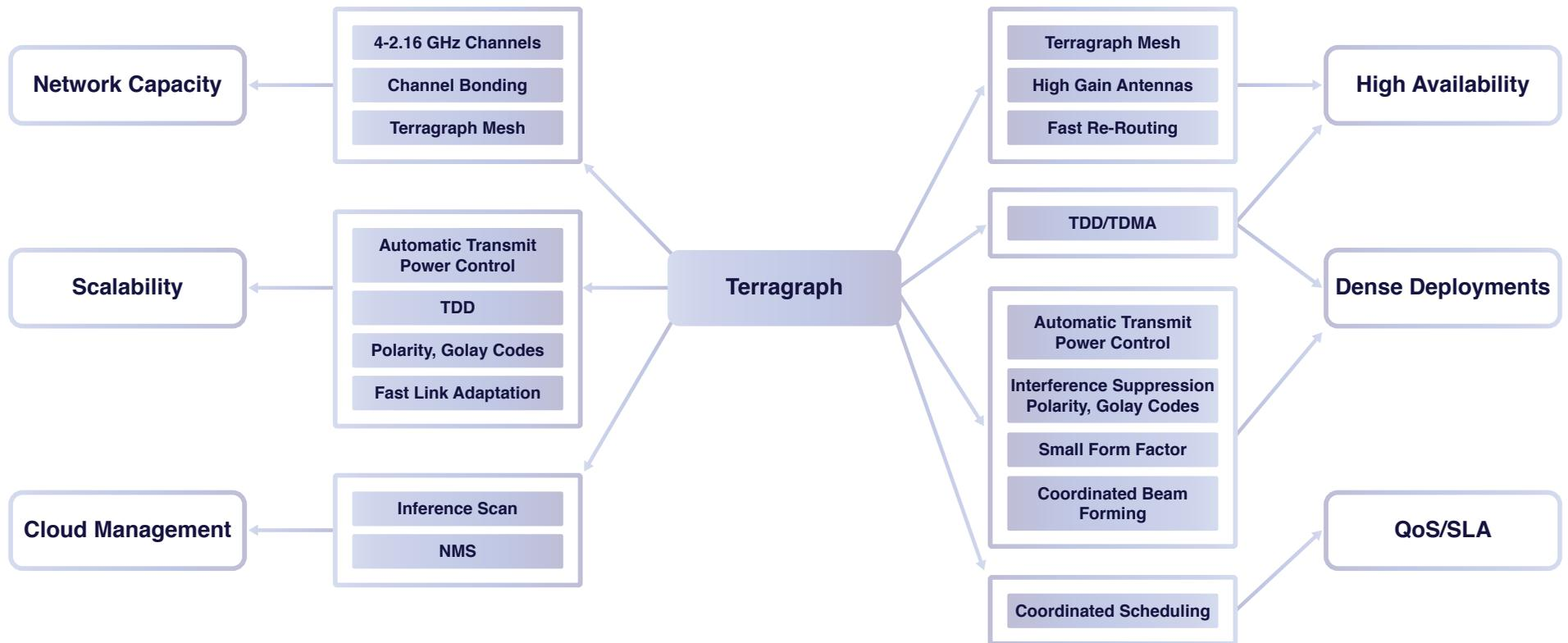
60GHz spectrum communication needs line of sight (LOS) and as a consequence is more prone to link outages. Terragraph mesh was developed to work around this challenge and to deliver high network level availability (e.g. > 99.9%). In the subsequent sections, we will describe how the Terragraph mesh network delivers high availability in a more robust and economical way than existing P2MP solutions.
