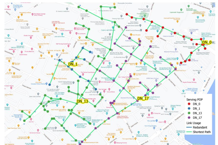
In the plot on previous page there is only one route from DN's to POP with no redundant links. The four different colors are based on the serving POP. The moment a Shortest Path link fails, The DN's on that chain will lose access to POP. In case of a failure of a POP, all DN in the cluster will lose connectivity.
